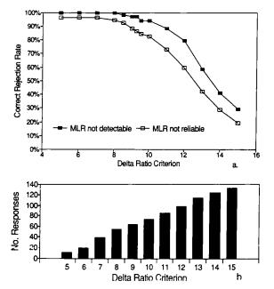
FIGURE 8. (a) The rate at which poor MLRs would be correctly rejected, given the delta ratio criterion. (b) The number of responses obtained with the delta ratio less than the criterion value. The optimum criterion is one that has a high correct rejection rate, but includes the maximum number of responses.
