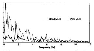
FIGURE 3. Frequency spectrum of EEG activity from C3-A2 during a period favorable for MLR and during an unfavorable period. Each spectrum is an average of the spectra of eight 10 sec epochs.
